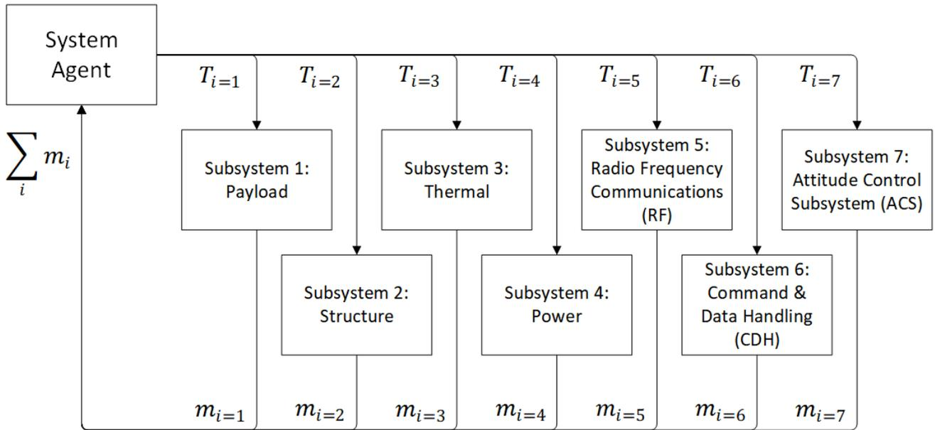
Fig. 1. The subsystem and system agents of the Agent Based Model, and the exchange of information between the agents during each design cycle
